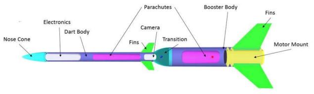
Figure 1: Cross section diagram of PR-3 "Thunder and Lightning"
