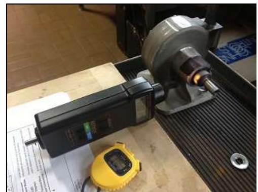
Figure 1: Optical tachometer and stopwatch positioned in the same video shot to enable video capture of turbine spindle experimental rotational velocity time histories for data analysis.
