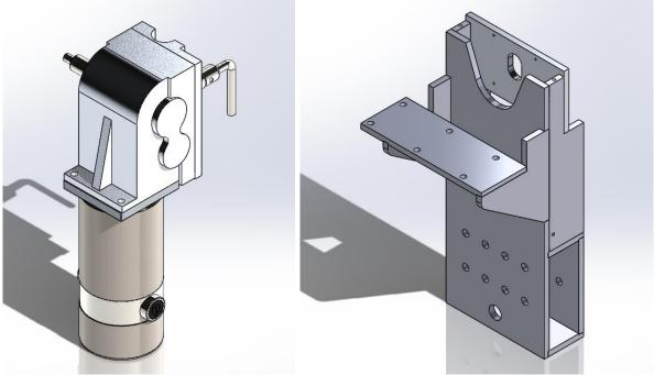
Figures 11 (left) and 12 (right). Motor and mount models.
