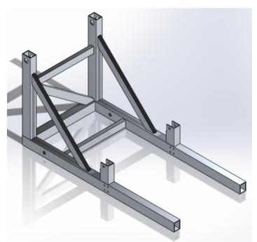
Figure 3. Final iteration of aluminum tube stock frame.
