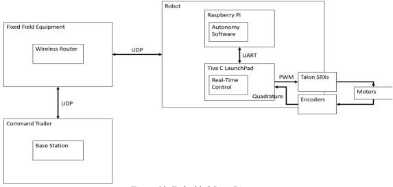
Figure 13. Embedded State Diagram
