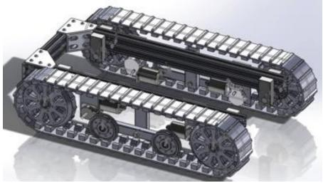
Figure 8. Older prototype powertrain assembly with SuperDroid wheels and treads.
