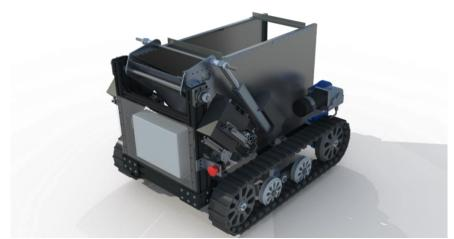
Figure 2. Rendering of prototype with 80-20 frame.
