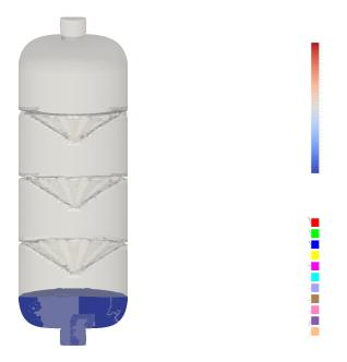
Figure 3: CFD simulations with anti-slosh baffles.
