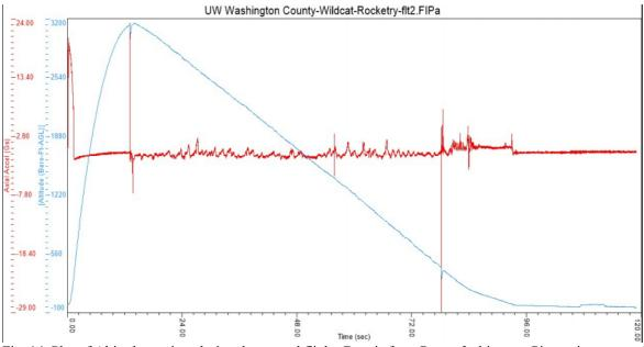
Fig. 14. Plot of Altitude vs. time during the second flight. Data is from Raven 3 altimeter. Picture is a screenshot taken from the Raven 3 data acquisition software by Dr. William Farrow of WSGC.
