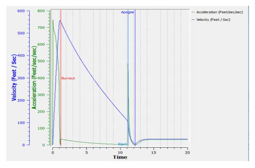
Fig. 8. Initial Rocksim Simulation with velocity and acceleration curves. Picture is a screenshot taken from Rocksim by a team member.
