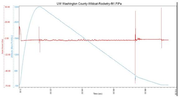
Fig. 12. Plot of Altitude vs. time during the first flight. Data is from Raven 3 altimeter. Picture is a screenshot taken from the Raven 3 data acquisition software by Dr. William Farrow of WSGC.
