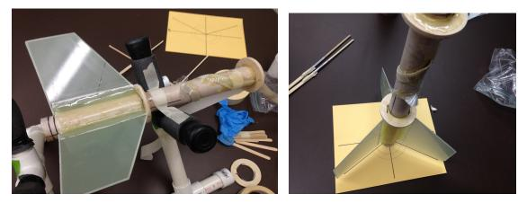
Fig. 4,5. Pictures of motor casing construction including the attachment and alignment of the fins. The fins were attached to the motor casing using epoxy. The lines on the yellow piece of paper were used to help space the fins as evenly as possible. Pictures were taken by a team member.
