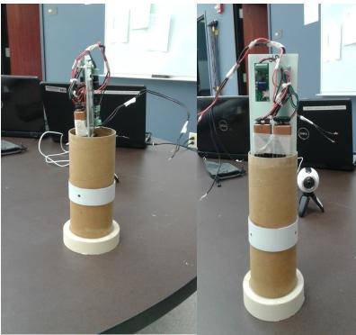
Fig. 2,3. Pictures of the electronics payload tube with the components tightened down and wired up on the tray. Pictures were taken by a team member.
