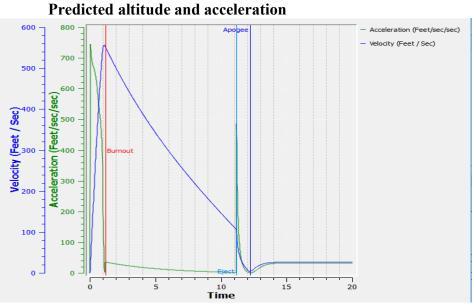
Fig. 10. An graph of predicted performance from an updated Rocksim Simulation after changes were made to the rocket design. Picture is a screenshot taken from Rocksim by a team member.
