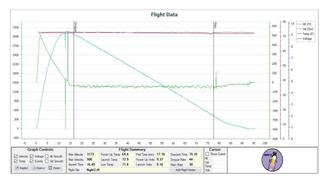
Fig. 13. Plot of altitude vs. time during the second flight. Data is from RRC3 altimeter. Picture is a screenshot taken from the program Missile Works Data Acquisition and Configuration Software by a team member.
