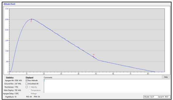
Figure 8: Stratologger data from the third competition flight. This flight had a tangled shock cord when main parachute deployed but it had no effect on decent rate.
