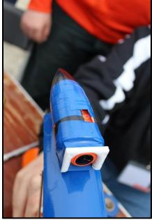
Figure 5: Improvised covering for the camera after the first flight
