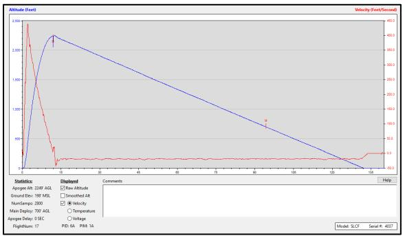
Figure 6: The Stratologger graph of the first competition flight of Focal point. This shows the anomaly of the constant descent rate indicating main parachute deployment at apogee.
