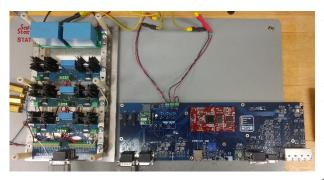
Figure 8, The AMDC connected to three inverter boards
