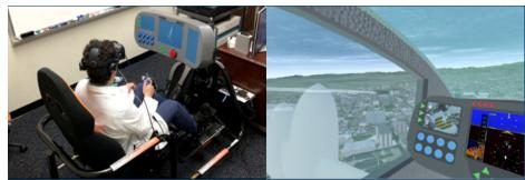
Fig. 8 The virtual and mixed reality environments of the UAM simulator
