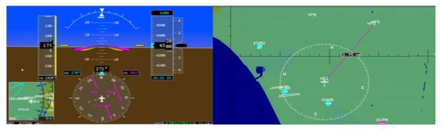
Fig. 3 (a) Primary Flight Display with Autopilot. (b) Multi-Function Display used for Navigation
