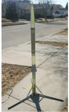
*Figure 6: Final rocket design with landing gear legs deployed*
