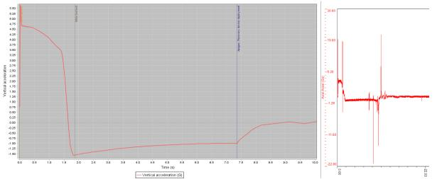
Fig. 8: Acceleration vs time simulation (left) and Raven data (right), showing a predicted maximum acceleration of 5.65 G, and an observed maximum sustained acceleration of 6.3 G.
