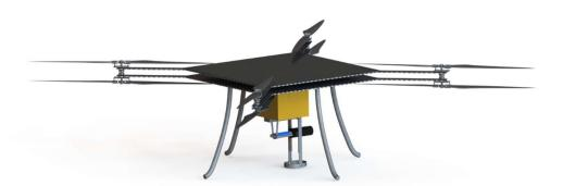
Figure 37: Drill mounted on stacked octocopter with drill in sample carrying position
