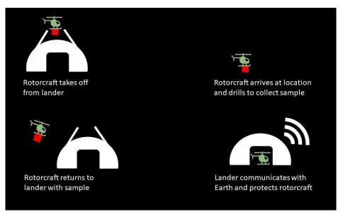
Figure 14: Polar Deposit Collection-CONOPS graphic
