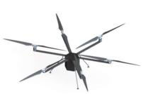
Figure 23: Overlapping Quadcopter
