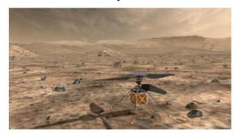
The Mars Helicopter [F2], sponsored by JPL, is part of the Mars 2020 mission as a technology demonstrator for extraterrestrial flight. The coaxial design has a rotor diameter of 1.21 meters with collective and cyclic control on both rotors and a maximum RPM of 2800. The helicopter has a
