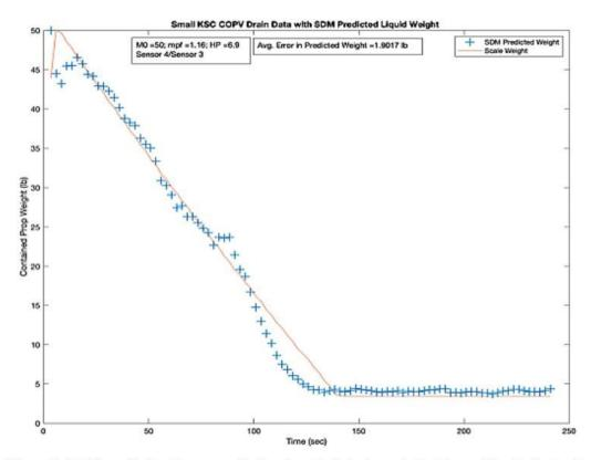
Figure 6. SDM applied to the composite linerless tank during a drain. The red line indicates the actual contained fluid mass and the blue marks indicate the SDM contained mass estimate.
