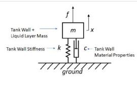
Figure 8. A visual depiction of what it physically means to model the tank as a single damped linear oscillator
