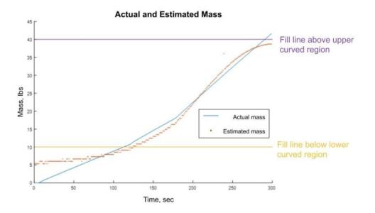
Figure 3. Actual and estimated mass of fluid within tank during a continuous drain test
