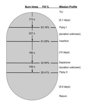
Figure 9. Mission Profile in relation to tank fill % - Dimensions to scale with Orion tanks
