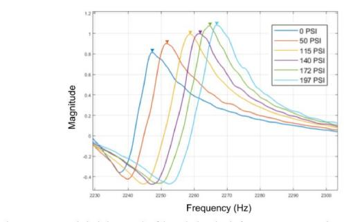
Figure 4. A graph depicting a mode of the tank changing in frequency as pressure changes and fluid volume remains constant.
