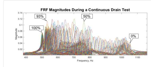
Figure 2. Processed FRFs, each averaged over 3 seconds in one second intervals during a continuous drain test
